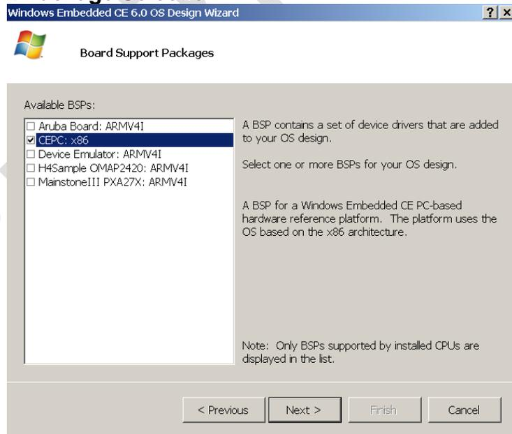
Figure 13: Board Support Package Selection Screen
