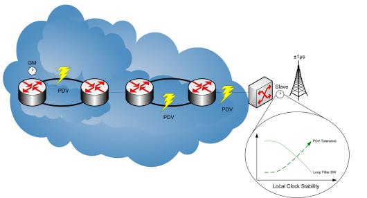
As Local Clock stability increases, the loop filter bandwidth can be reduced and PDV tolerance goes up
