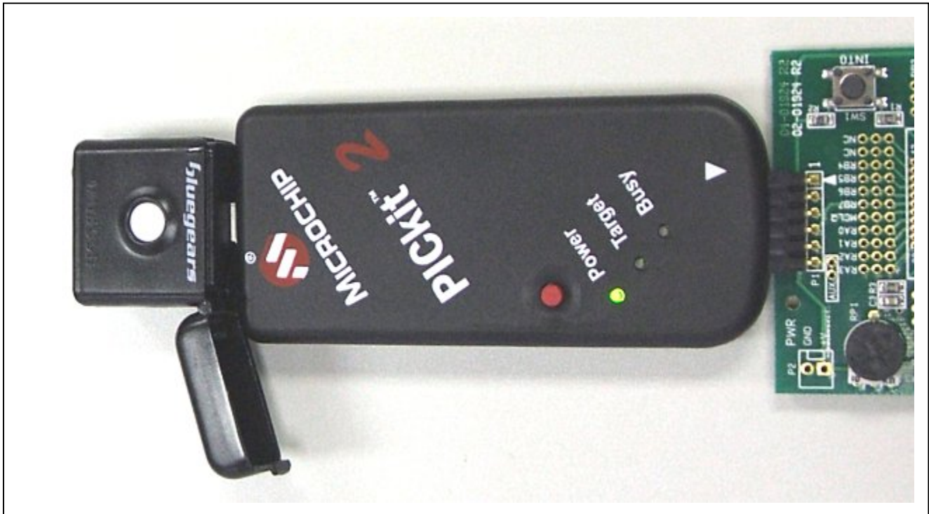
FIGURE 2-2: B-MOBILE POWERING PICKIT 2 UNIT FOR PROGRAMMER-TO-GO OPERATION
