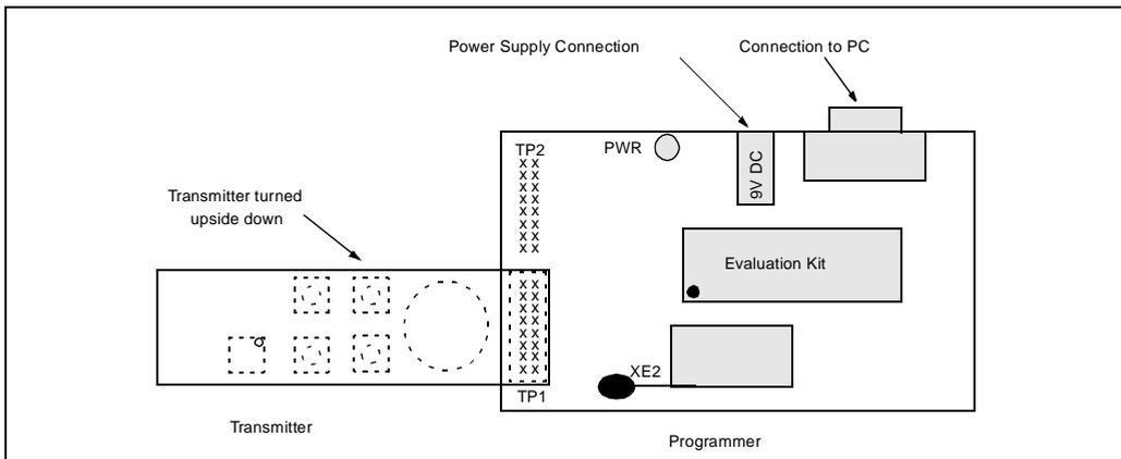
Figure 6.4: Programming the Demonstration Transmitters
