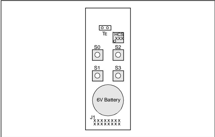
**Figure 4.1: KEELOQ Demonstration Transmitter**
