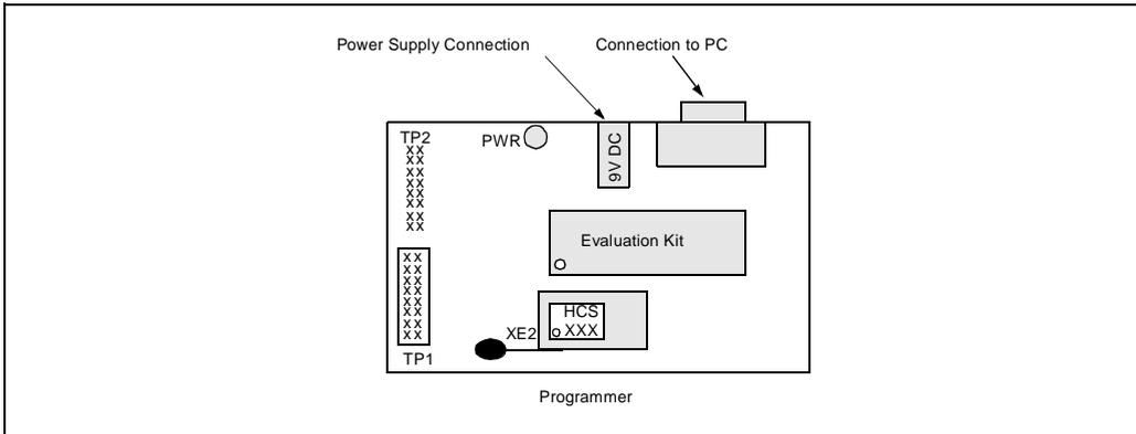
Figure 6.3: Programming an Encoder DIP
