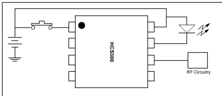
**Figure 3.1: Typical KEELOQ Transmitter Circuit**
