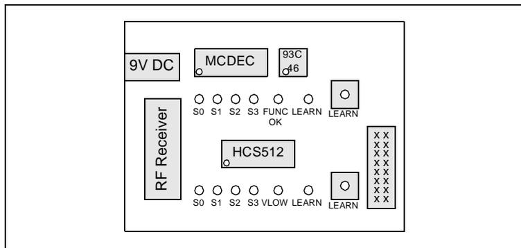
Figure 5.1: KEELoQ Decoder Demonstration Board
