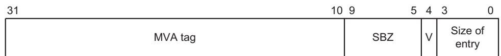
Figure B-3 Rd format for accessing MVA tag of main or lockdown TLB entry
