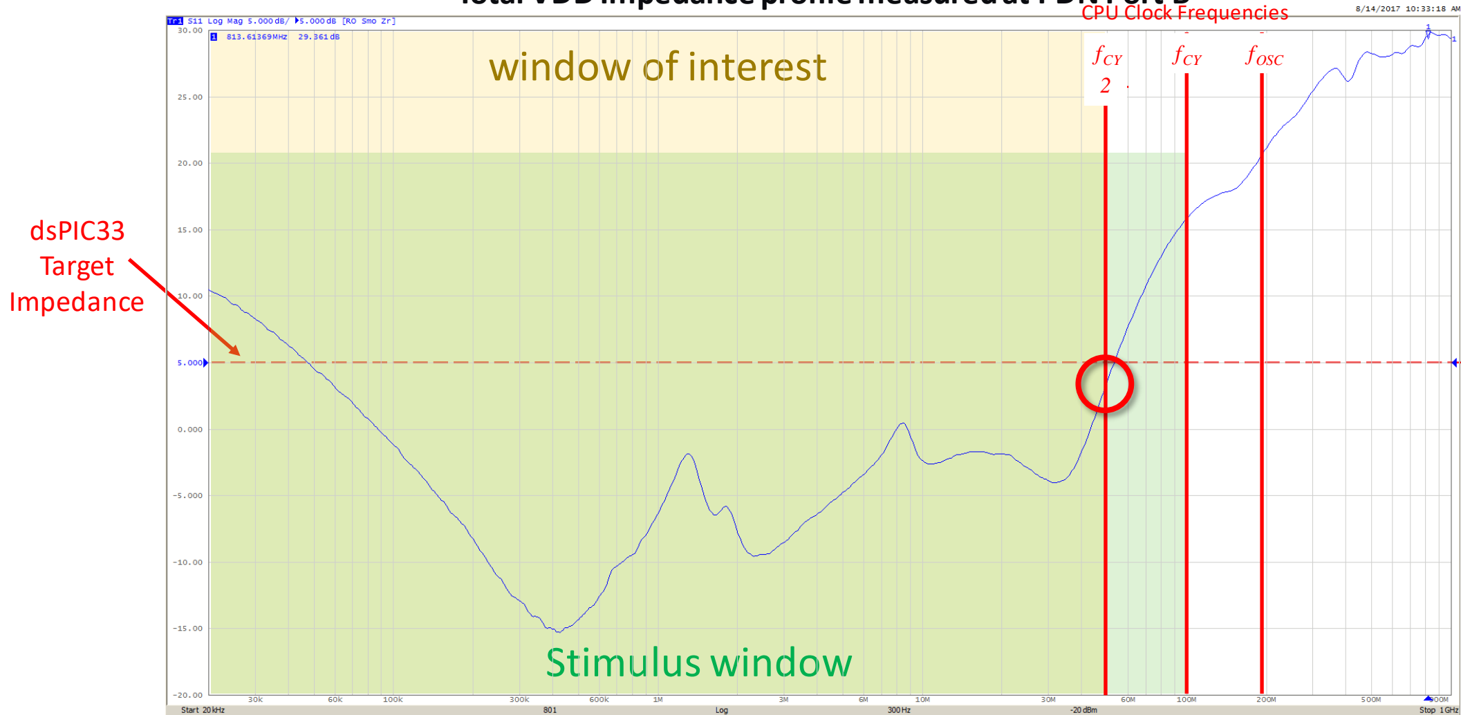
Total VDD Impedance profile measured at PDN Port B
