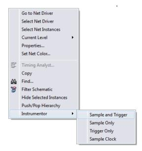
When selected, the instrumentation is automatically applied to the open instrumentor view.
