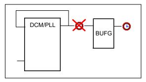
You can also select the sample clock from the RTL window by right-clicking on the watchpoint icon in the source code display and selecting Sample Clock from the popup menu. The icon for the selected (single-bit) signal changes to a clock face as shown in the following figure.
