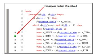
Once a breakpoint is instrumented, the instrumentor creates trigger logic that becomes active when the code region in which the breakpoint resides is active.
