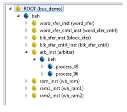
Single clicking on any element in the hierarchy browser causes the associated HDL code to be visible in the RTL tab display.
