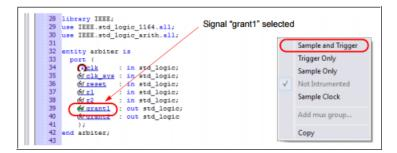
The TCL Script window at the bottom displays the Tcl command that implements the selection (signals add -iice {IICE} -sample -trigger {/beh/arb\_inst/grant1} and the results of executing the command.
