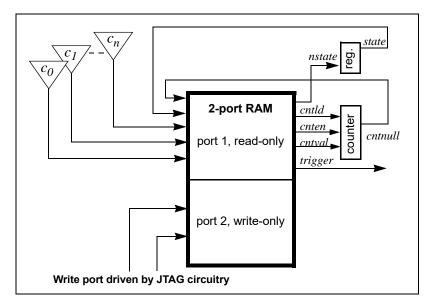
The implementation of the RAM table is identical to the implementation of the sample buffer (that is, the device buffertype setting selects the implementation of both the sample buffer and the state-machine RAM table).
