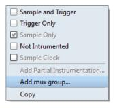
In the Add mux group dialog box displayed, select a corresponding group by checking the group number and then click OK to assign to the signal or bus to that group. A signal can be included in more than one group by checking additional group numbers before clicking OK.
