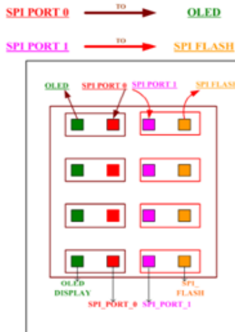
JP8 Jumper settings for SPI flash
