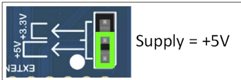
FIGURE 1-7: ATMBUSADAPTER-XPRO DEFAULT SUPPLY JUMPER SETTING
